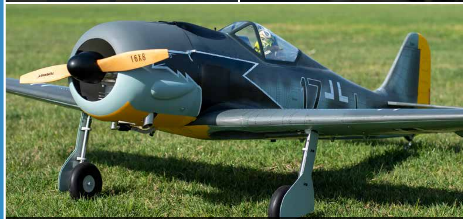
23cc gasser spinning 16x8 prop provided the perfect powerplant combination.
